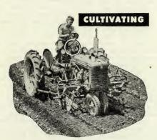
Front and rear cultivator units or left and right sections on this Farmall C may be lifted independently or their depth adjusted by Farmall Tauch-Cantrol.
